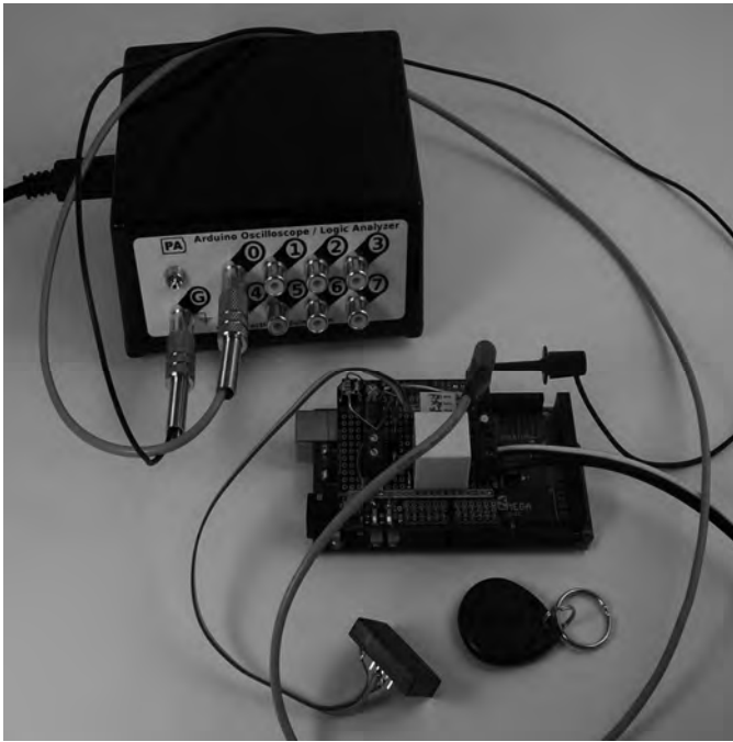
Figure 11-10. Connection to a circuit under test
