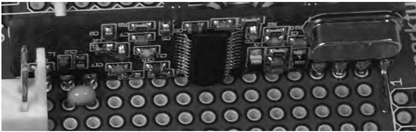
Figure 13-8. RXB1 receiver mounted on shield
